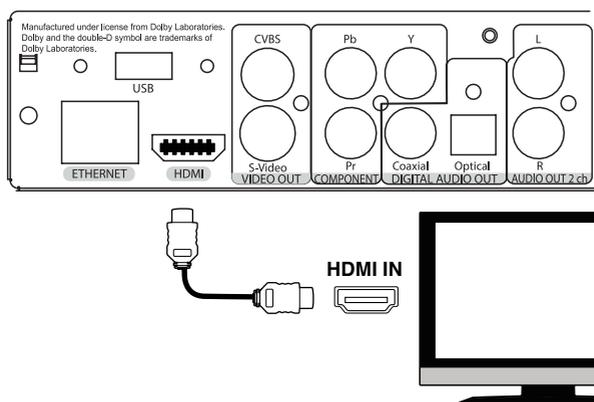
Since Dune BD Prime is designed first of all for playback of high definition (HD) video (up to 1080p), the best way of signal transmission from player to a TV set or projector is the HDMI interface. In this case, video and audio streams are transmitted in digital form, without losses, allowing enjoying excellent picture and sound. It is recommended to connect the player to any compatible equipment using original DUNE HDMI cable (option).
